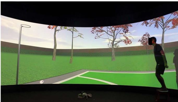
**Figure 1** — The custom-built VR game. Participant stood on the 30-cm block and performed a maximal drop vertical jump. If the sensor (located in middle of image) detected the projected frontal plane knee angle was  $<9^\circ$ , the ball (pictured on the left) would enter the hoop and participants would score a goal. If the knee angle detected  $\geq 9^\circ$ , then the ball would miss the hoop. VR indicates virtual reality.
