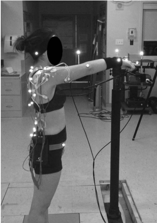
**Figure 1** — Experimental setup of a subject standing at the repetitive pointing apparatus.
